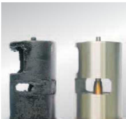
Since EGR valves do not soot themselves, it is essential to search for the causes of soot formation.
