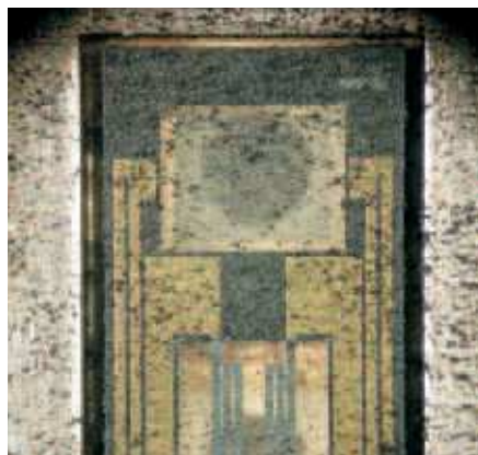
Salt and dirt may damage the sensor of an air mass sensor – they will at least falsify the measurements, which in turn could affect exhaust gas recirculation.
