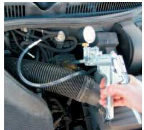
Whether dealing with pneumatic EGR valves or an electro-pneumatic pressure transducer, as in this case: The function can easily be tested using a vacuum hand pump.
