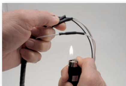
Heat it using a lighter until it shrinks and completely covers the connection
