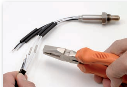
Crimping the butt-type connector.
