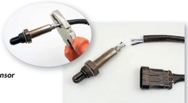
Disconnect old Oxygen Sensor from vehicle and cut the wires close to the Sensor's body
