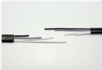
Do staggered cuts in wires from new Oxygen Sensor and in wires from old connector
