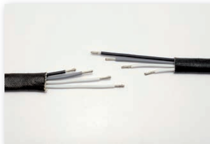
Stripping off approximately 1/4" of insulation from the end of each wire
